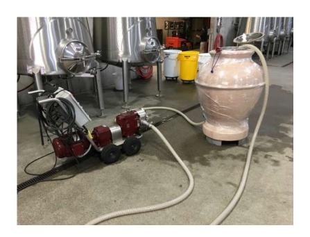
Use a spray ball similar to the one above that sprays evenly and can operate at low pressures. Create a recycling system with two hoses and a pump set at a low pressure.
