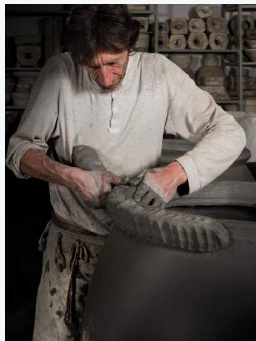
Colombino technique being applied to make a classic amphora.
